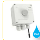
TEV-3 Thermostat for regulation of heating (cooling), adjustable range 5 to 35°C (41°F to 149 °F), external sensor NTC, output contact 16 A, control potentiometer and indication on panel. page 139
