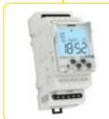
TER-9 2 temperature inputs, 2 outputs 8 A changeover/SPDT, 6 functions, in-built time switch clock, LCD with back light, galvanically sep. supply voltage AC 230 V or AC/DC 24 V, 2 MODULE. Temperature range: -40 °C to 110 °C (-40 °F to 230 °F). page 136
