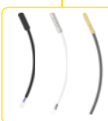
TC, TZ, Pt100 External temperature sensors for thermostats in lengths 3m, 6m, 12m (9.9', 19.7', 39.4') TC/TZ: thermistor NTC 12 kΩ/25 °C (77 °F) Pt: element Pt100 (only TER-3G). page 145
