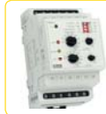
TER-4 Wide and accurate range of setting -40 °C to 110 °C (-40 °F to 230 °F) in ten ranges in one device, fine temperature setting. 2 inputs for NTC sensor, 2 outputs 16 A changeover/SPDT, additional function (memory, hysteresis, indication of faulty sensor). Supply: AC 230 V or AC/DC 24 V (galv. separated). page 134
