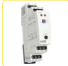
TER-7 Monitoring heating of motor winding in range given by resistance of in-built PTC thermistor(1.8-3.3 kΩ), additional function (memory, reset), output contact 2x 8 A changeover/DPDT, supply: AC/DC 24-240 V. page 133
