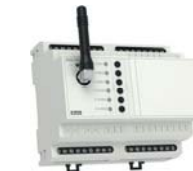
RFDEL-76M Universal dimmer, 6-channels – 6 x 150 VA
